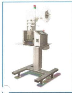
AZCO Corp's SUR-PAK<sup>TM</sup> Pouch Dispenser is designed for ease of use and reliability. The unit comes on an adjustable height stand with castors for easy integration into packaging lines. The unit is self-threading and will feed, cut, and place the pouches directly into a product or packaging line. The sachets or pouches can be either in roll form or continuous bandolier form. The SP-4D dispenses pouches up to 89 mm/3.5 in. wide and 6 mm/0.25-in. thick at speeds of up to 100 pouches/min.
